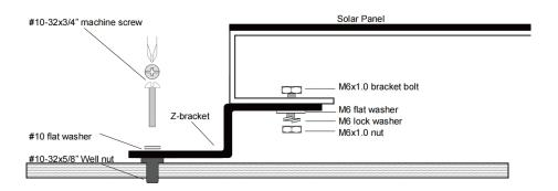
Gently insert the well nut into the drill hole. Be careful not to push the well nut flange completely into the holes. Make sure the flange is flushed on the roofline.Before attaching the panel to the roof, a film of caulk can be laid between the RV roof and the Z-Bracket. Even though the well-nut provides a watertight bond, this provides additional sealant.
